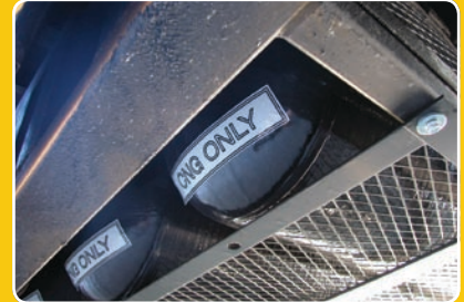
Five CNG tanks (65 diesel gallon equivalent).
