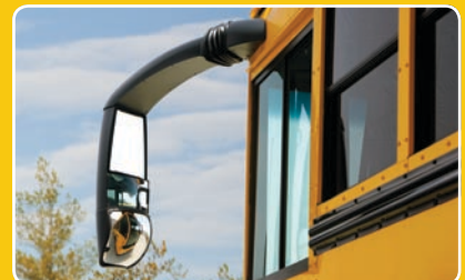
Flat and convex integrated mirrors improve rear-view visibility.
